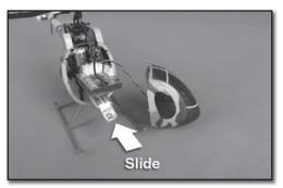
Slide the flight battery into the battery compartment.
