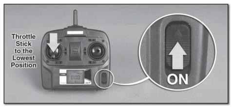
☐ Move the throttle stick to the lowest position and then turn the transmitter on.
