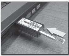
Plug the battery into the charger. The indicator light will start flashing, indicating that the battery is being charged. Once the battery is completely charged, the charge indicator light will stop flashing. Disconnect the battery from the charger. Under normal operating conditions, the battery may take up to 60 minutes to recharge.
