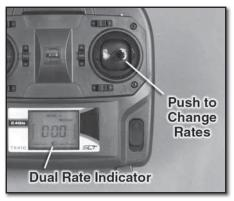
The dual rate switch provides dual control rates for the cyclic and tail rotor controls. Please use the low rate until you become accustomed to your MD-530. Change the dual rate using a quick push of the right stick. To adjust the dual rate, push and "hold" the right stick and move the throttle stick to the desired percentage. Release the right stick to set.
